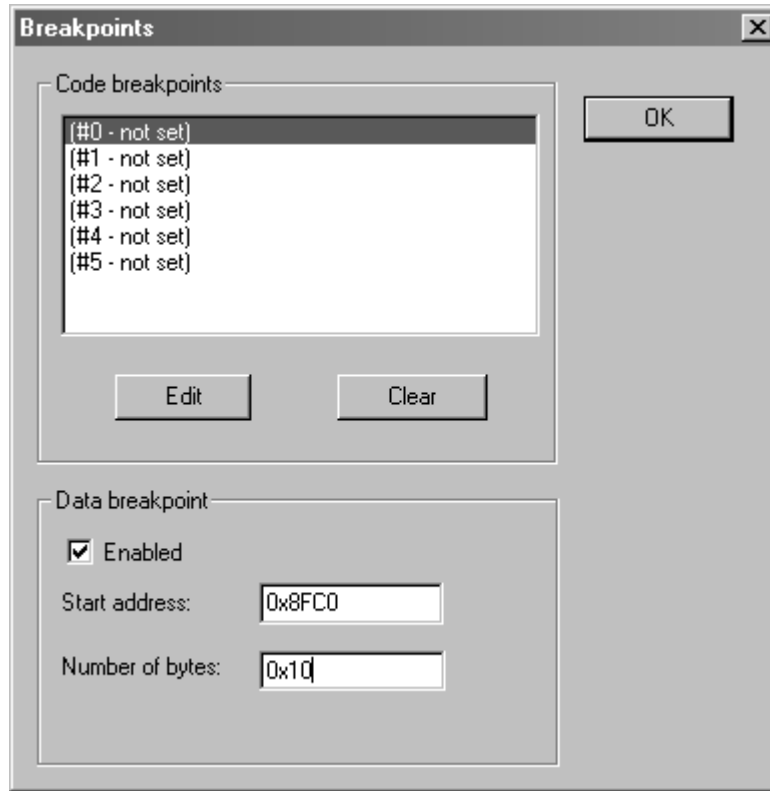
Figure 5.6 Setting a Breakpoint
